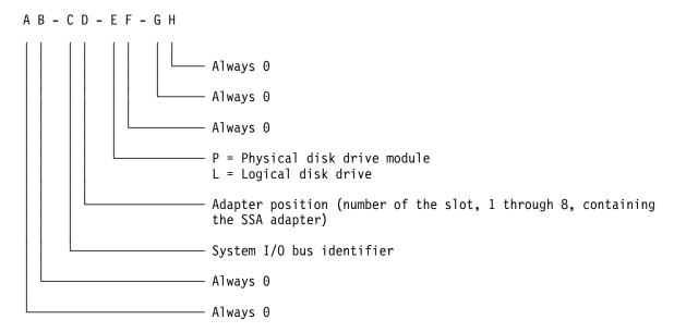
The location code shows only the position of the SSA adapter in the using system and the type of device that is attached. Use a service aid to find the location of the device (disk drive module). For more information, see "SSA Service Aids" on page 7-30.
